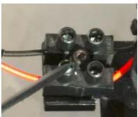
4. Remove the temperature sensor cable.
