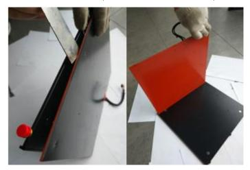
8. Prepare a new heated bed and adhere it to the insulated plate. *Note*: Pay attention to the location of the breach.
