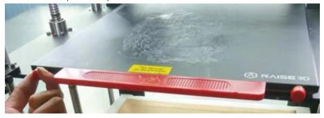
3. Remove the heated bed power cable by loosening the two screws on the left of the terminal block with a small flat head screwdriver.
