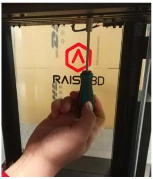
6. Clamp the nuts with pliers, use a 2mm hex wrench to remove the 12 nuts from the screws, pull the screws out of the heated bed, and separate the insulated plate from the heated bed.
